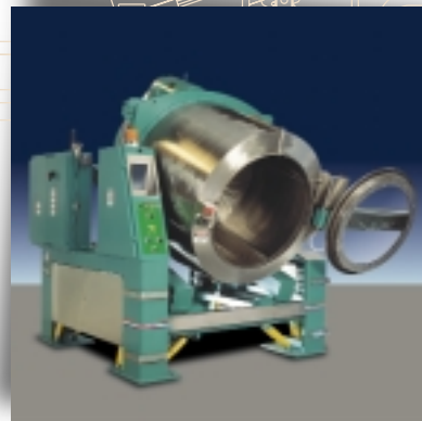
All machine functions are controlled by the combination of a PLC and a TouchScreen microprocessor formula control used as the operator interface.
