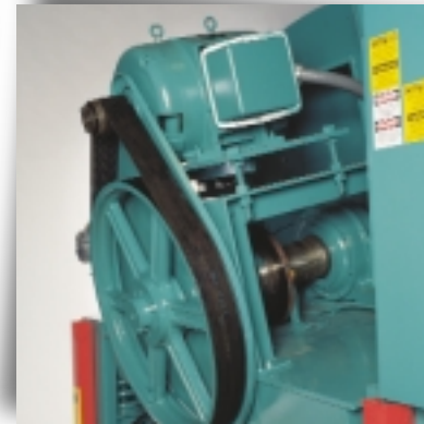
Brim's simple variable speed electronic single motor drive precisely powers the washing and extraction cycles, and eliminates high maintenance components such as multiple motors, clutches, and intermediate transmission devices.
