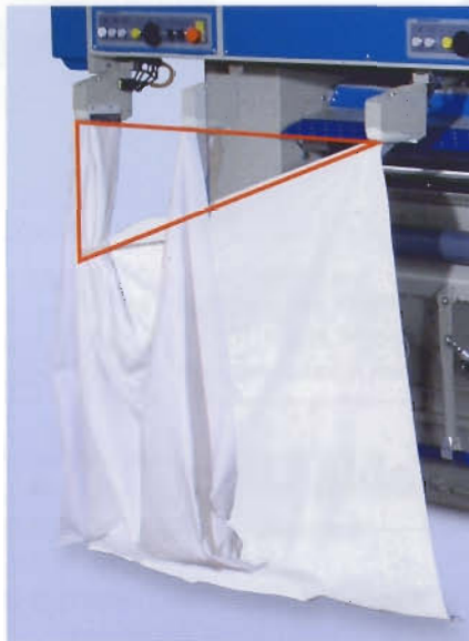
Spreading principle: Measuring followed by spreading
