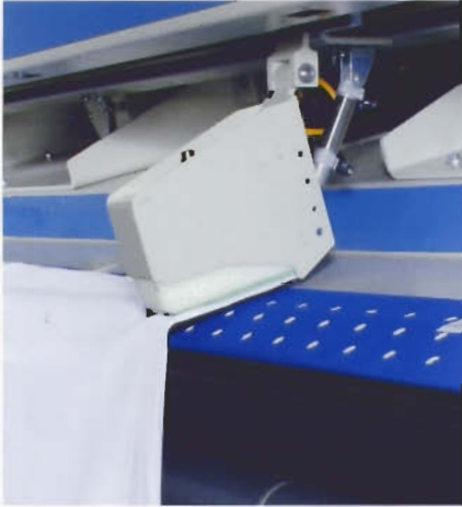
Transfer position of the clamp onto the vacuum transfer bar
