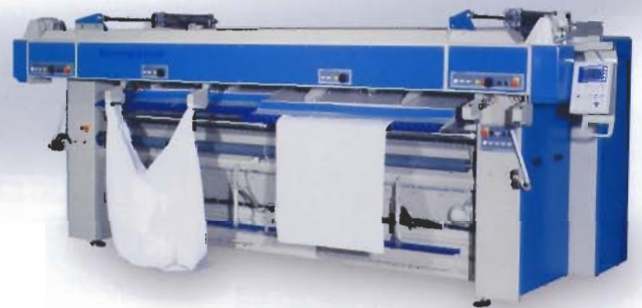
First lane: clamp feed from the lane centre Second lane: manual feeding onto the vacuum transfer bar
