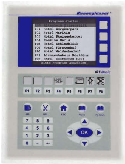
Control panel model IBT enables production, programming and fault finding modes.
