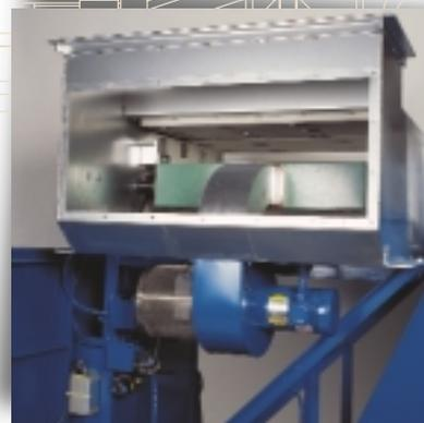
An Eclipse forced draft ribbon burner, fed by an IRI-compliant modular gas train that requires no vent valve, provides the 74/78G's heat source.
