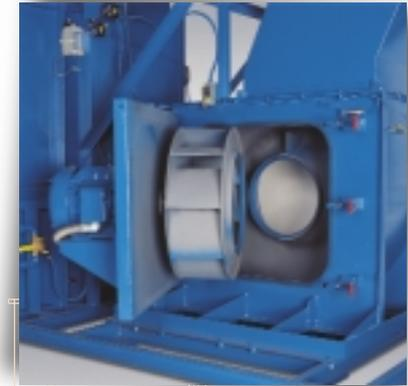
The Brim 74/78G Dryer incorporates a backward-inclined fan design, which moves a high volume of air at a low velocity, thus reducing noise and providing evenly distributed airflow for maximum moisture removal.
