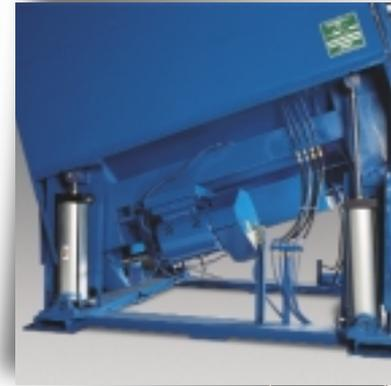
As with all Brim products, heavy-duty construction and ease of maintenance are hallmarks of the 74/78G, from a solid steel base frame that supports the basket housing to a convenient swing-out blower that makes lint removal from the fan blade a quickly-performed task.
