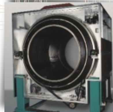
The Dryer's basket is rotated by a smooth belt drive connected to a constantly adjusting motor plate assembly.
